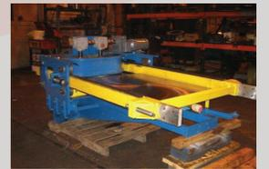
Oxy Fuel Cutting of Lower Die Shoe with Three Scrap Ramps
